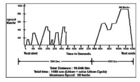
Fig. 3 Driving Cycle for emission measurement
