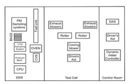
Fig. 2 Equipment layout for Emission testing
