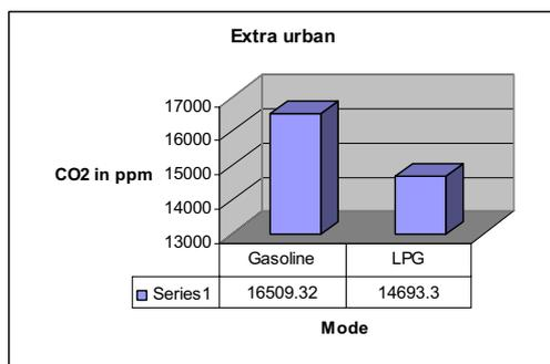
Fig. 11 Graph of CO<sub>2</sub> in extra urban cycle
